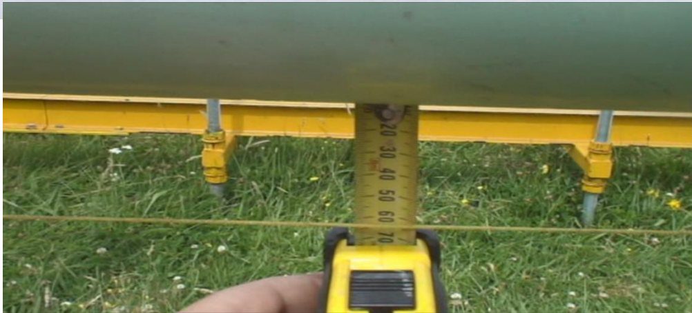
When manually measuring sweep the tape measured 6.1-6.2 cm of sweep The Forest Bucker scanned sweep at 6.1 cm.
